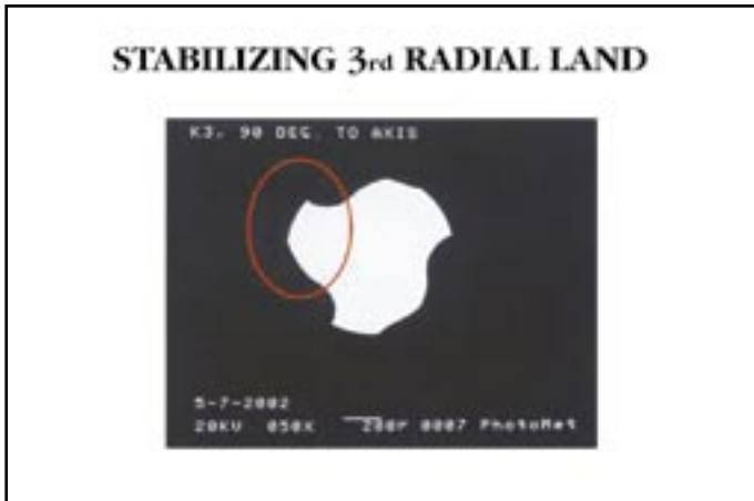
Fig.21.3.The K3 has a series of three radial lands when viewed in cross section, with relief behind two of the lands. The feature reduces friction on the canal wall and prevents overengagement and helps keep the file centered.
